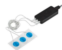
EMG curve is smooth and precise thanks to an external preamplifier.
